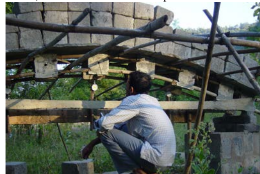
h) Creep experiment on Bamcrete Bow Beam
