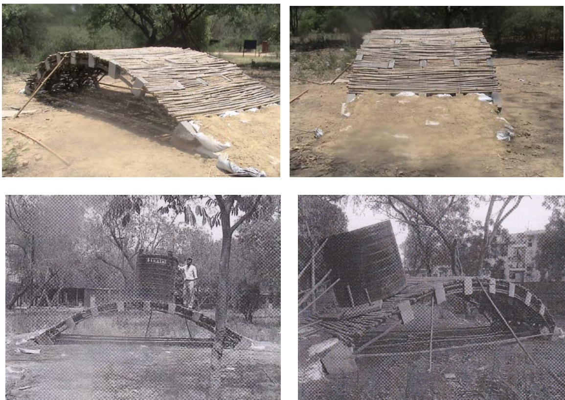
Fig. 13: Bamcrete Bridge and its loading
