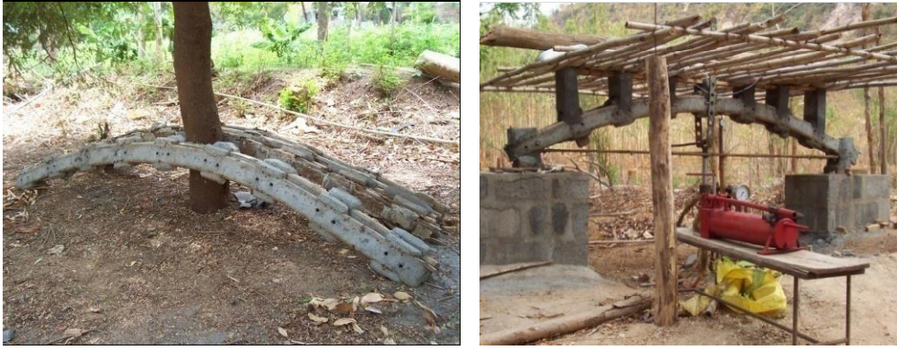
Fig. 4: Half Split Concrete Infilled Bow Beam and its experiments
