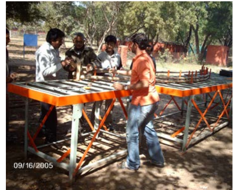
Fig. 7 Work Bench for Bending Bamboo
